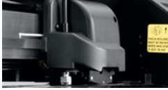
Fig. 4.11-4: Cutting head with sensor and tangential knife
