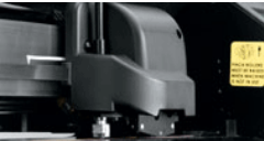
Fig. 11.4-1: Cutting head with sensor and tangential knife
