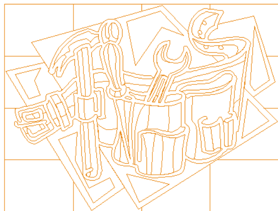
Fig. 12.1-5: Result of the output with weeding lines - objects not! cut
